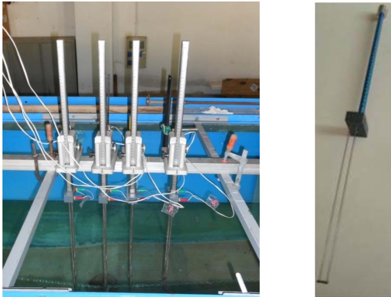
Fig. 31. Resistive wave gauges: large (left) and small (right)
