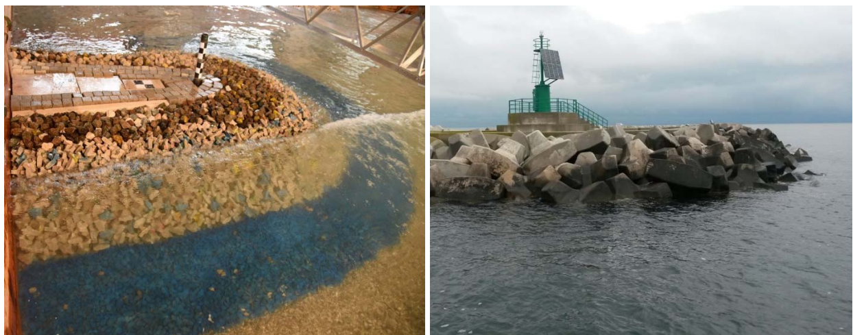
Fig. 25. Roundhead stability 3D test
