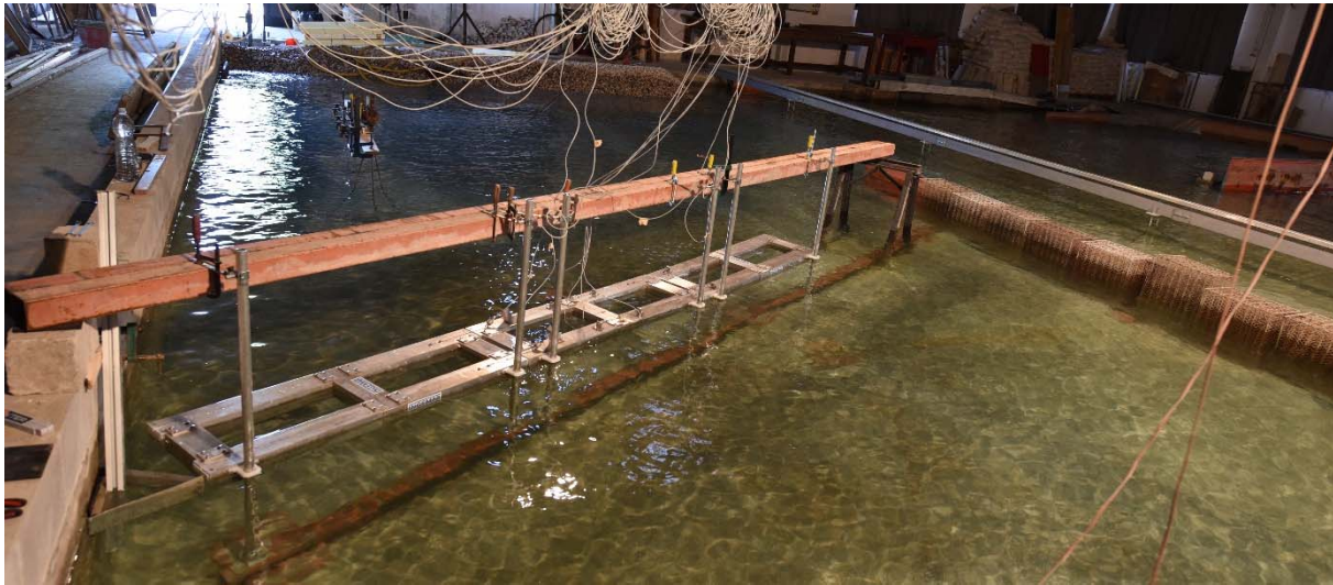
Fig. 30. Floating structures (evaluation of loads)
