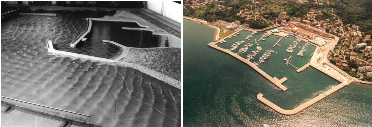
Fig. 20. From the model (left) to the construction (right)
