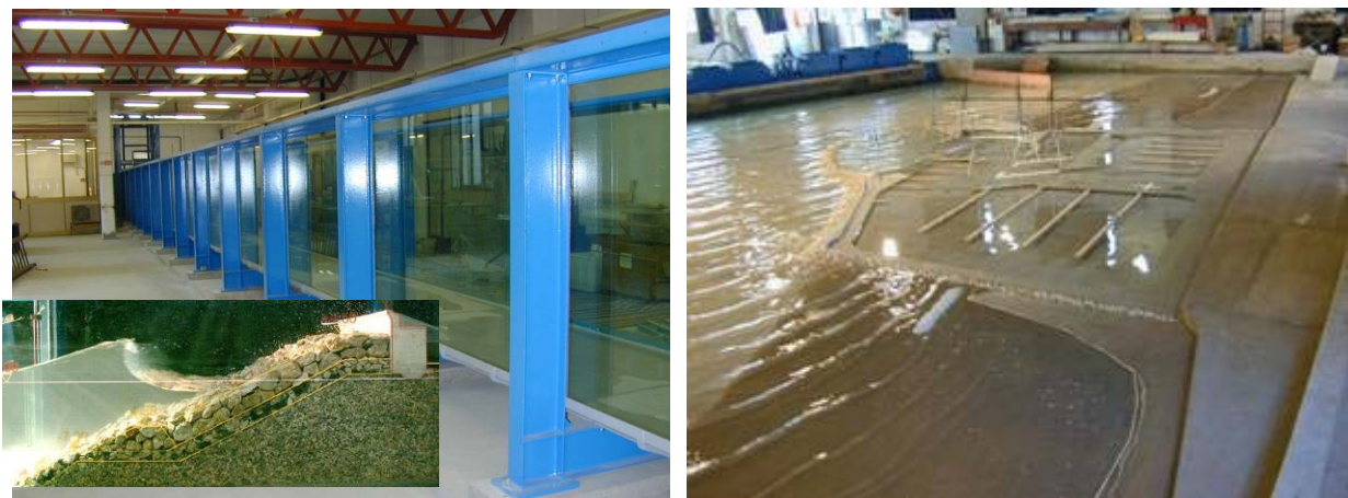
Fig. 1. Wave flume (left), wave basin (right)
