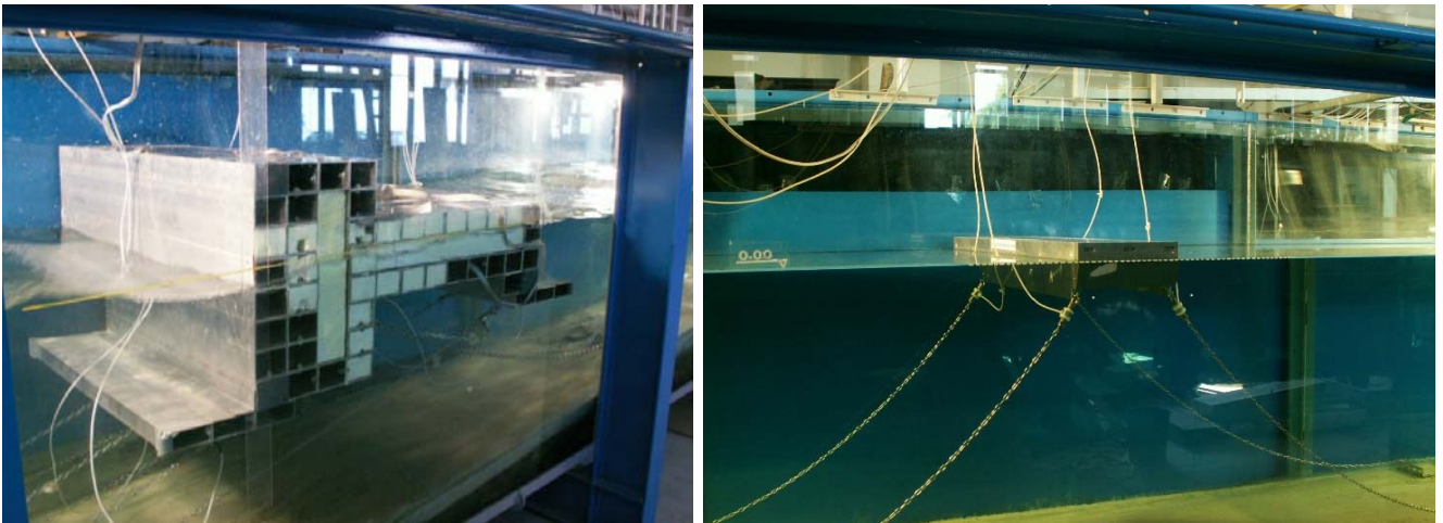
Fig. 9. Floating breakwaters (wave reflection, wave transmission and loads)
