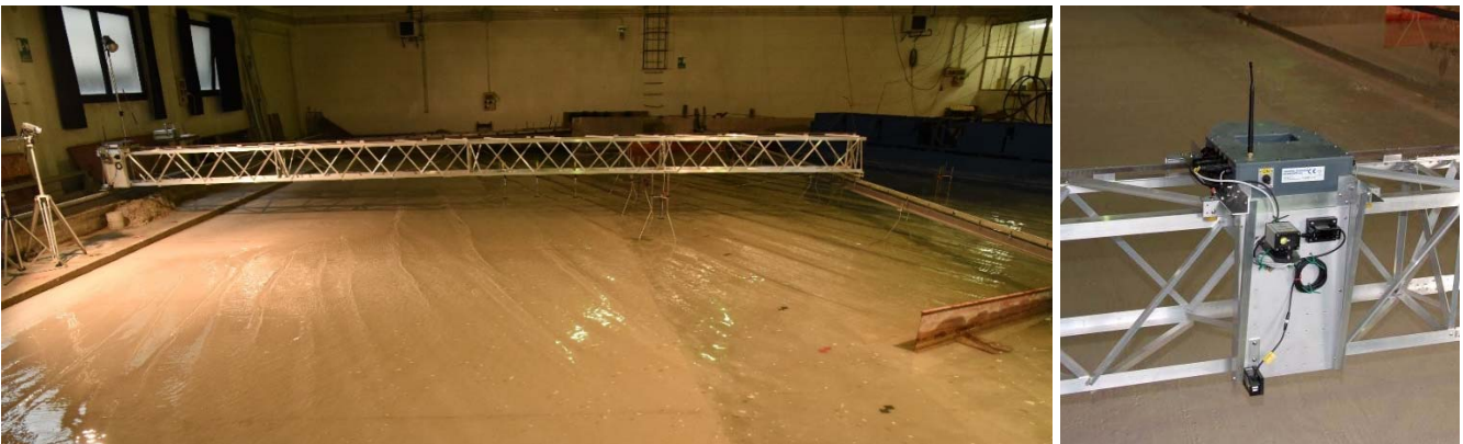
Fig. 32. 2D bed profiling system
